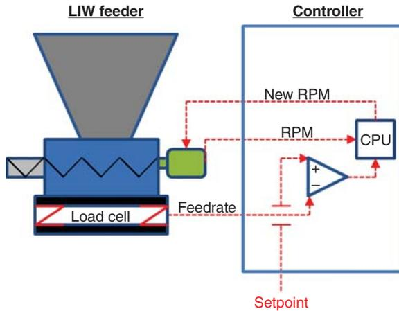
**Figure 12.1** Diagram of the main components of a loss in weight feeder. A volumetric feeder is mounted on a load cell with a feedback controller monitoring and controlling the feed rate.
