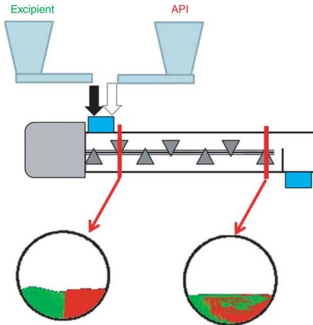
**Figure 12.4** Illustration of radial mixing phenomenon in a continuous tubular blender along the blender length. Each radial cross-section in the blender exhibits the same arrangement of components over time but subsequent cross-sections do not.
