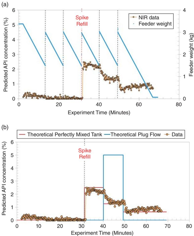
**Figure 12.2** (a) RTD response of a K-Tron KT-20 feeder to a pulse of tracer material (acetaminophen). The solid lines show the weight of the material in the feed hopper as a function time. The spikes indicate hopper refills. (b) Fit of the data to standard CSTR and PFR models. It can be observed that mixing inside the feeder mimics a perfect CSTR, characterizing substantial back mixing.
