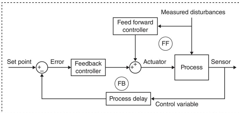
**Figure 12.9** Combined feedforward/feedback control.
