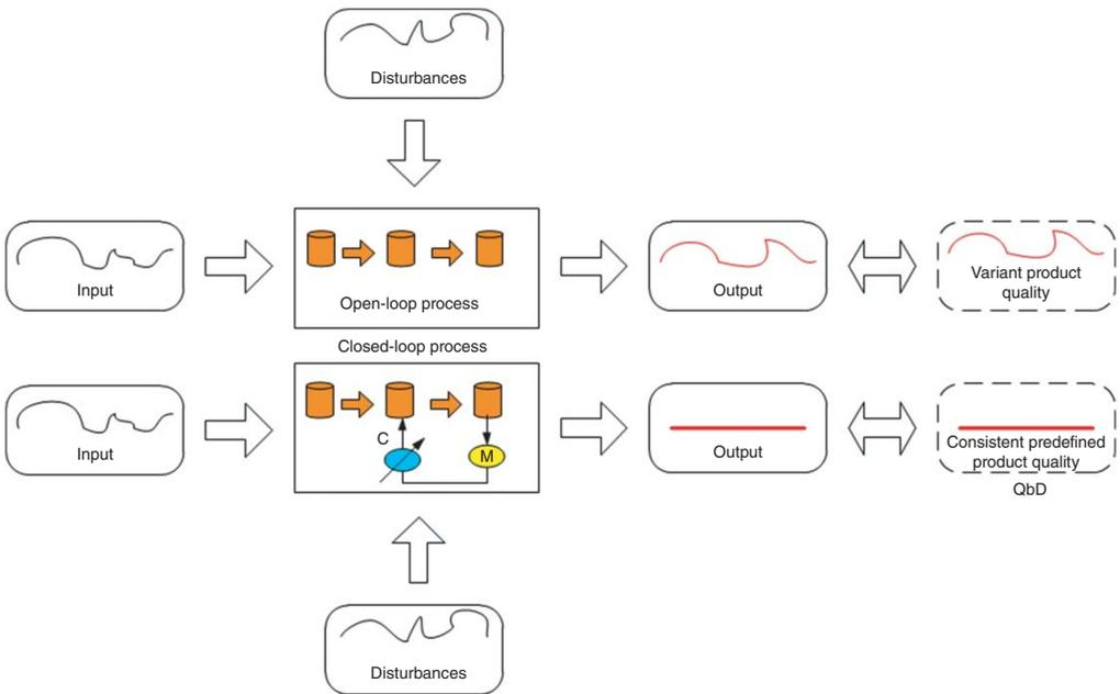
**Figure 12.8** Illustration of closed-loop and open-loop operation (adapted from [50]).
