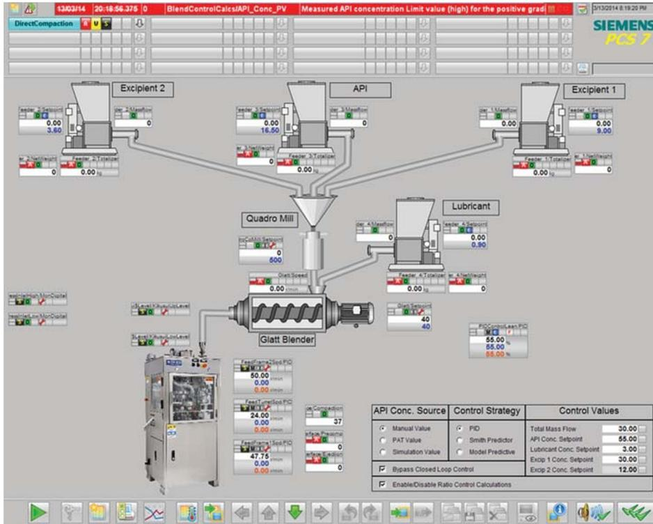
Figure 12.13 Plant operating and control user interface.
