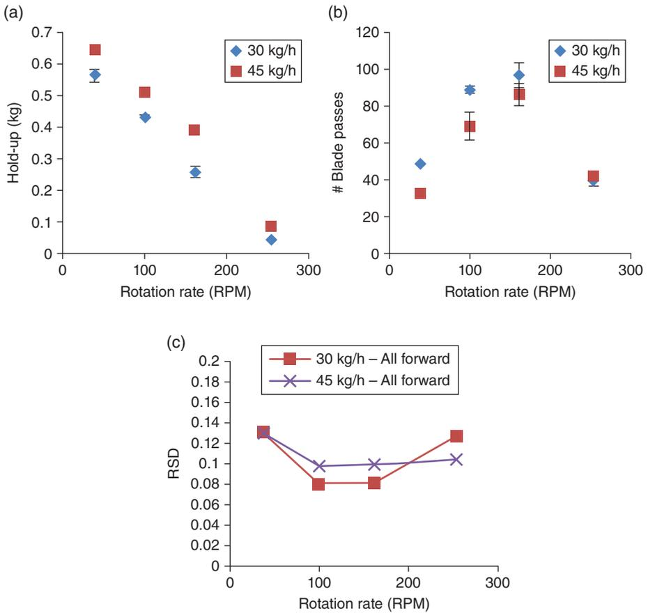
**Figure 12.3** Effect of impeller speed on (a) mass-holdup, (b) number of blade passes, and (c) relative standard deviation of the active concentration in the outlet stream for an all forward blade configuration.
