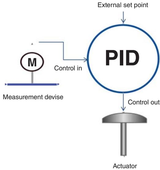
**Figure 12.10** Integration of a control loop with the process model.
