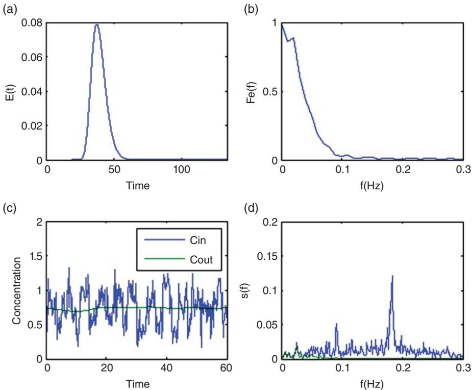
**Figure 12.5** Noise analysis of KT-20; worst case noise coupled with worst case RTD for filtering noise. (a) Normalized RTD of the blender. (b) Filtering ability of the blender. (c) Concentration in versus predicted concentration out after axial mixing in blender. (d) Noise spectrum of the raw feeder (upper line) versus effective frequency filtering done by the blender (lower line).
