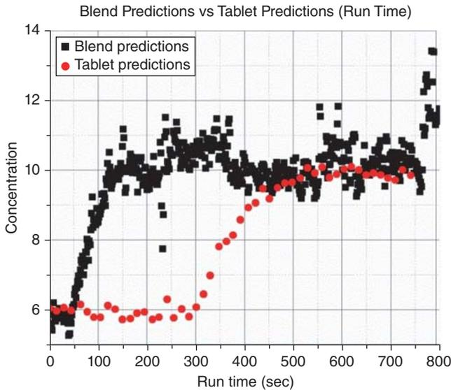
**Figure 12.7** At time 0, feed ratio was changed from 6% APAP to 10% APAP. The series of squares is the in-process spectra of the material post the blender. The series of circles represents NIR measurements on tablets sampled at the exit. It takes about 9 min after the perturbation having exited the blender to manifest itself into tablets.
