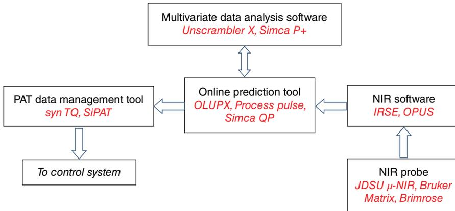
**Figure 12.11** Flow of communication from a sensor to the data management tool. Examples of each tool from different vendors are also given.
