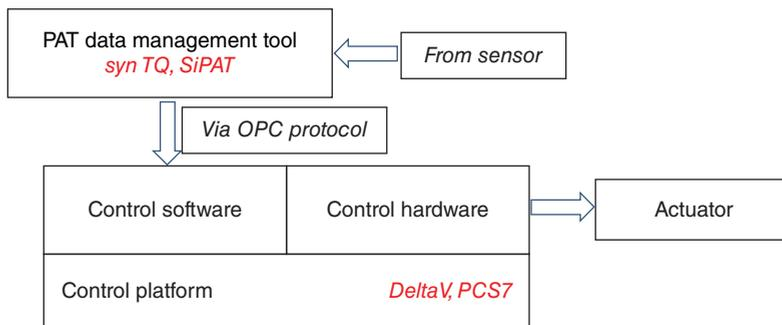
**Figure 12.12** Flow of communication from the PAT data management tool to the actuator.
